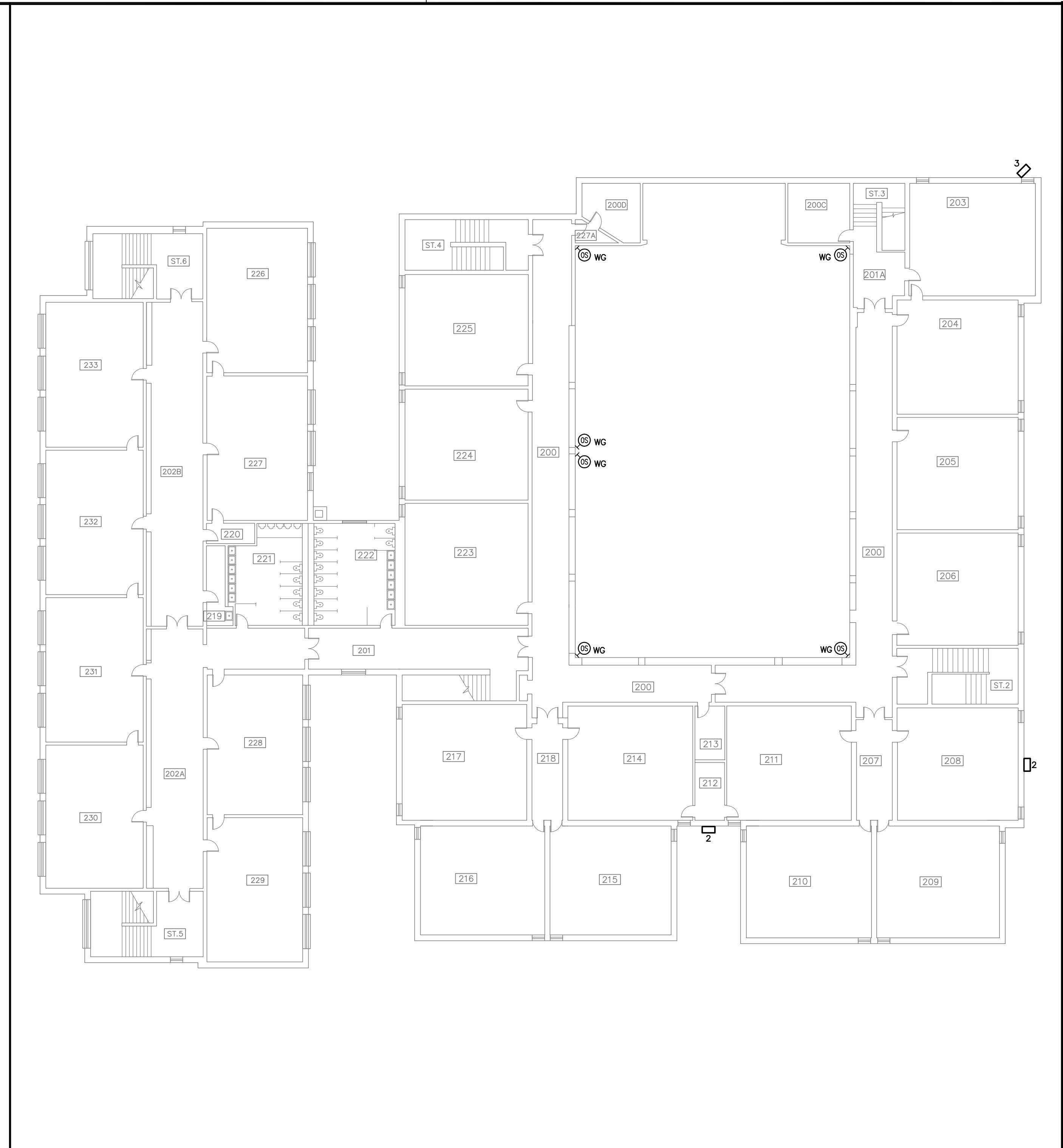
3 SECOND FLOOR PLAN - LIGHTING E-1 1:200
