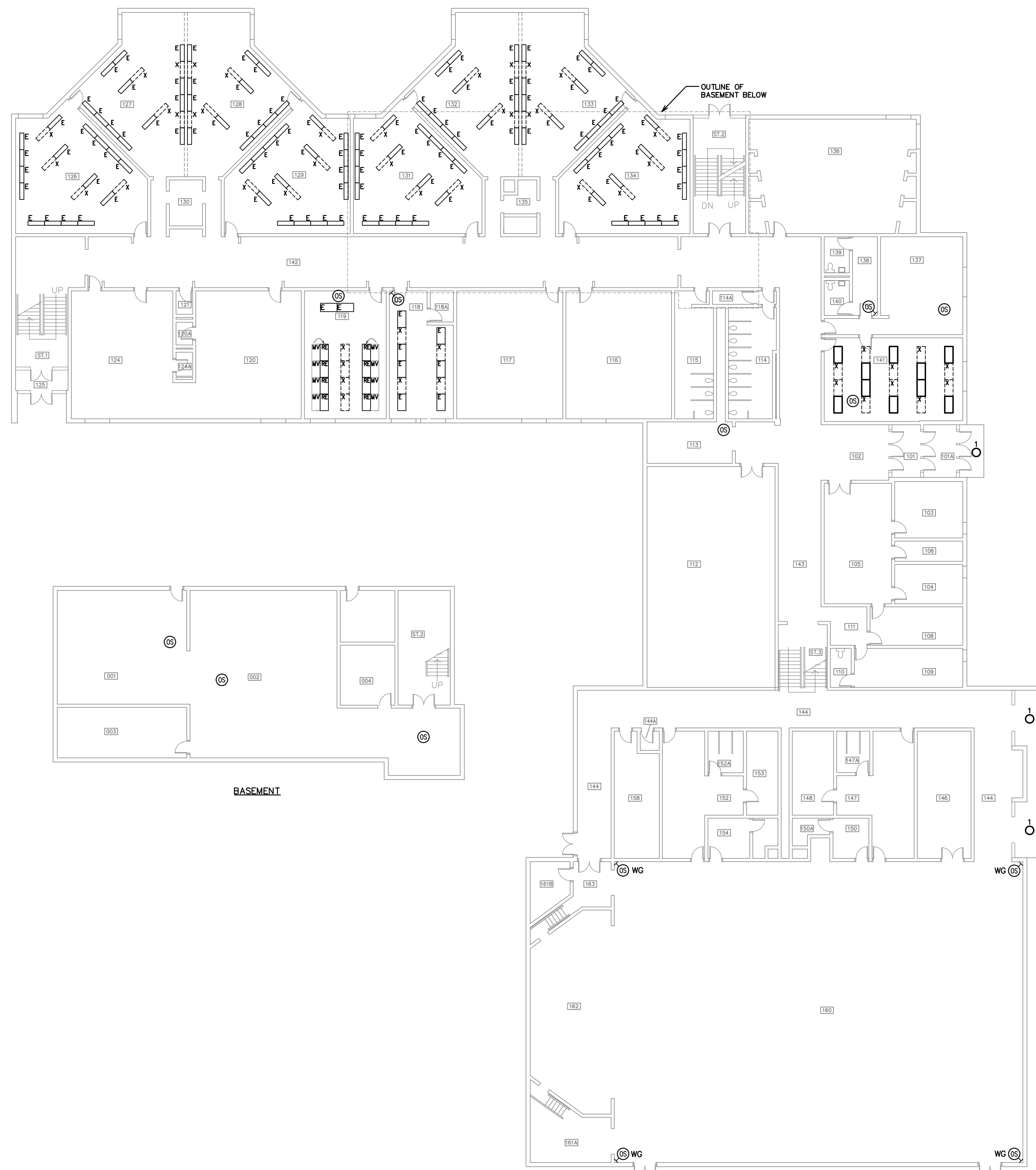
1 E-1 GROUND FLOOR & BASEMENT PLAN - LIGHTING 1:200
