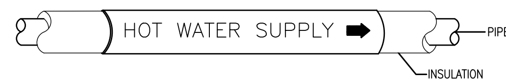
4 TYPICAL PIPE IDENTIFICATION MH501 NTS
